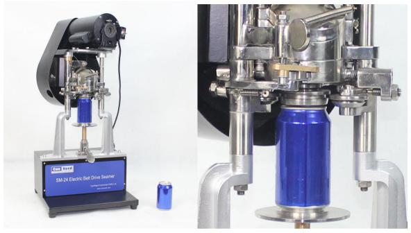
"CanNeed-SM-24 Electric Belt Drive Seamer" (Desktop model) enables the users to do more lab tests. Such as, adjusting some technique, enhancing the products quality, test the empty cans and free ends, to insert a temperature logger into a can before running a temperature monitoring.
